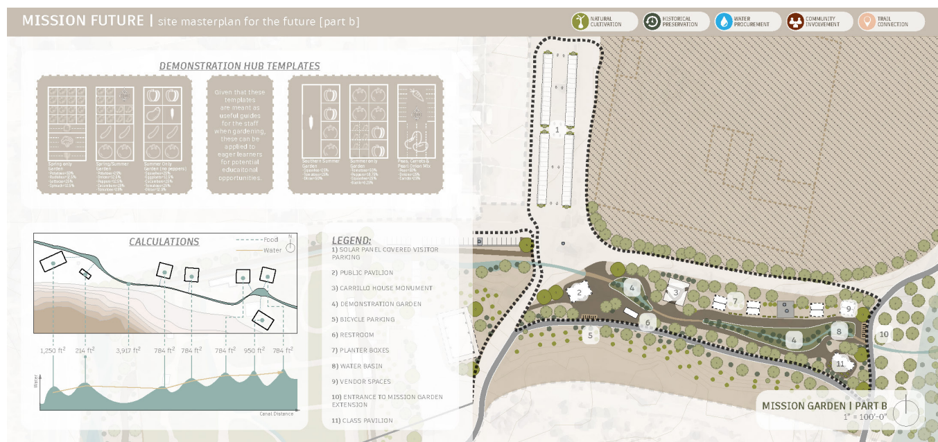
FIGURE 2: Water harvesting calculations for Mission Garden (author: ARCH 410f Spring 2021 students Rico Lizama and Bo Su and author)
